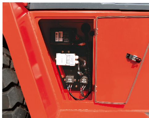
Independent integrated electric cabinet
