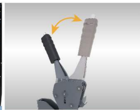
Ratchet type hand brake
