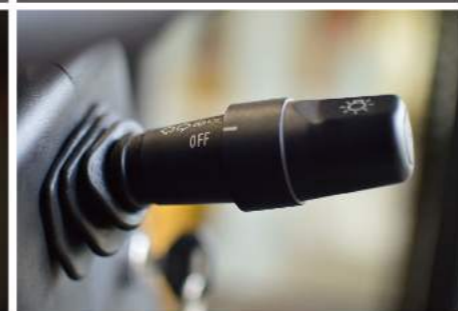
Integrated light switch
