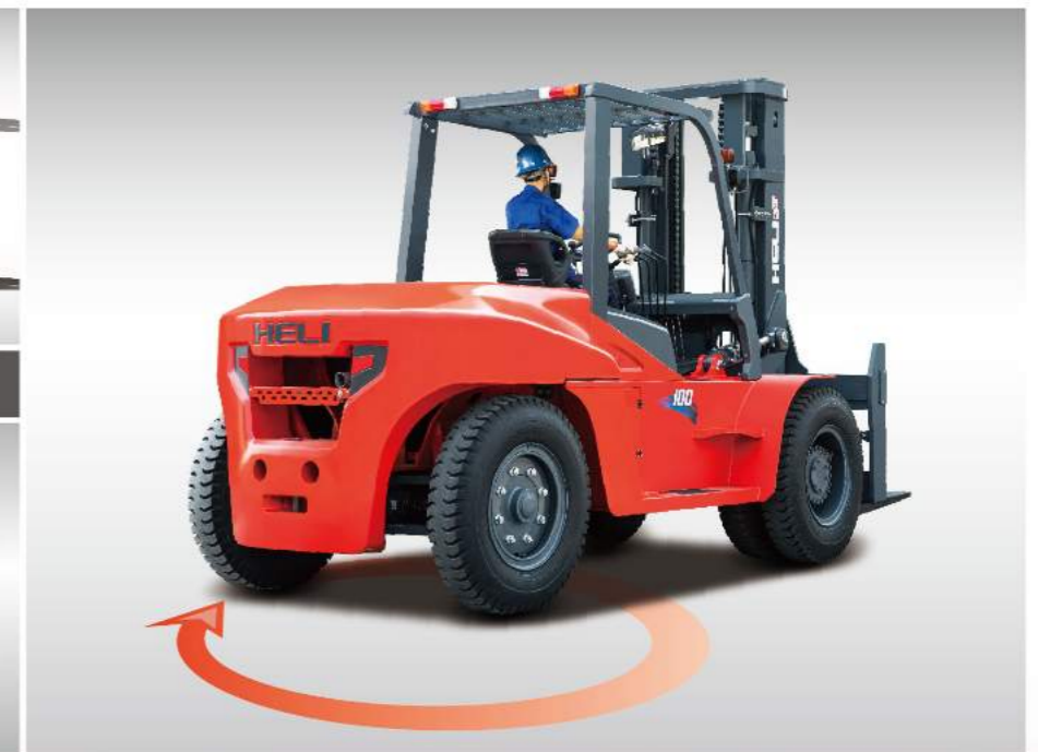
Large steering angle axle is equipped to get smaller turning radius.
